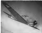
ZERO agile World War II fighter (here in U. S. markings) carried two cannons, two machineguns, weighed less than 6,000 lb.
